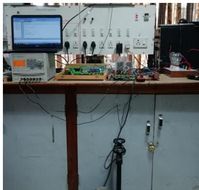
Implementation of Impedance-source Inverter (ZSI)
